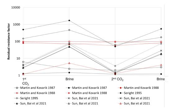
Fig. 2—WAG after CC/AP gel placement in sandstone. The x-axis starts at the first CO<sub>2</sub> injection. Multiple corefloods are presented in most papers (duplicate paper listings). The RRF values are provided in the appendix, Table A-2.
