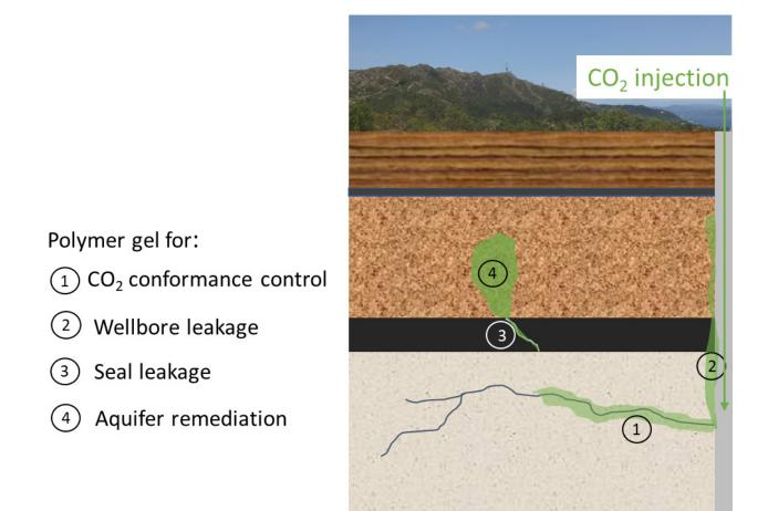
Fig. A-1—Polymer gel has been implemented for  $CO_2$  conformance control (1) and researched as a means to remediate wellbore (2) or seal (3) leakage, or  $CO_2$  leakage to and in an over-lying aquifer (4).
